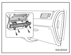
1) Remove the four screws from the filter cover located below the glove box.
